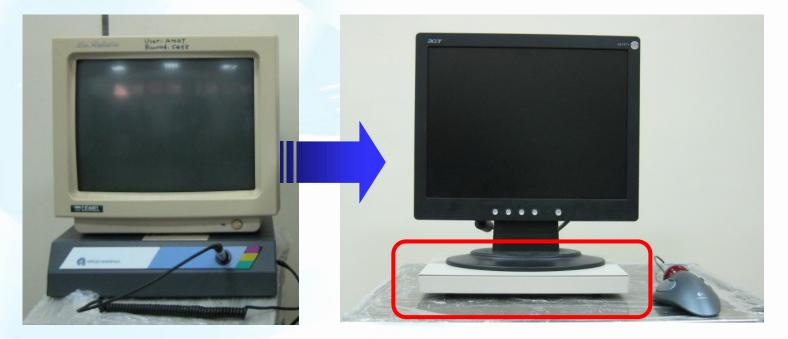
L X W X H = 302mm X 215mm X 35mm (Including port and feet) Size is designed to sustain a monitor (Can be customized)
